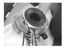
Using a pair of channel lock pliers that are large enough to grab the outer circumference of the valve flange on the outside and gently break loose the valve from the nut, by turning the outer valve counter clockwise. Also be sure that you take care not to damage the inflatable material.
