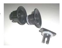
It is a rather simple procedure to replace a valve. At the factory, we install valves very tight since the inflatable material will take a set, or be permanently deformed by the ridges that are molded into the valve flange where they compress the fabric. The valve will be hard to break loose at first but can be easily turned with a pair of pliers.
